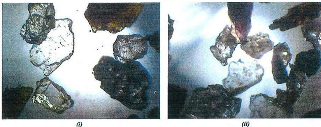
Fig. 4 Mgf X40 (+150 microns): Angular to sub-Angular grains of quartz, mica flakes and lithic fragments. Note some of the grains are coated with iron oxides.
