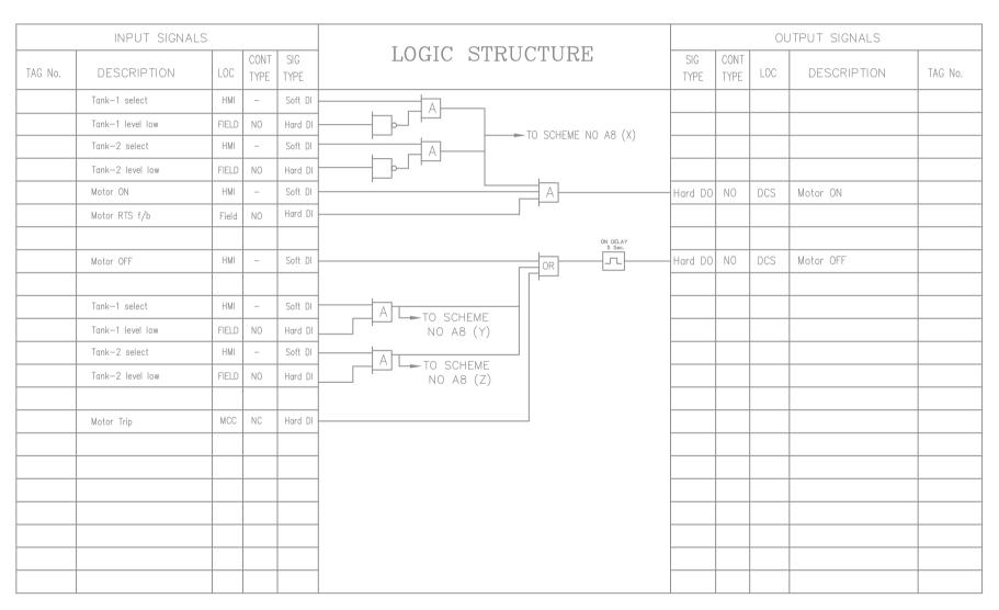
THIS LOGIC IS APPLICABLE FOR HRSG FILL PUMP.
