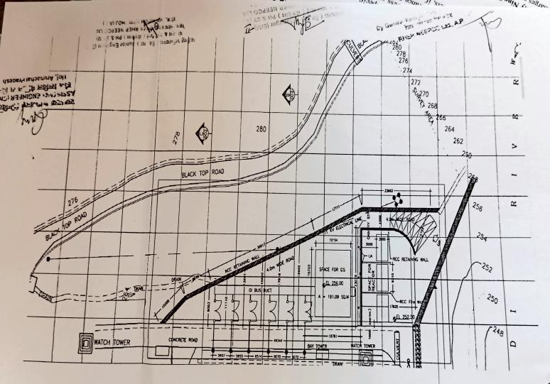
Proposed Protection Wall for 400kV GIS Bay Extension at RHPS, A.P. Total Length of Wall =50 RM
