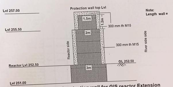
C/S details of protection wall for GIS reactor Extension
